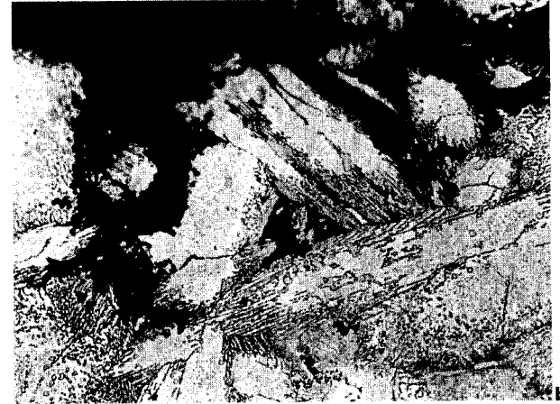
8 Microsections ( \times 500 ) of corroded NAB after coupling to Z100 in (a) natural sea water and (b) chlorinated sea water (area ratio 1:10), etched electrolytically in 1% chromic acid
