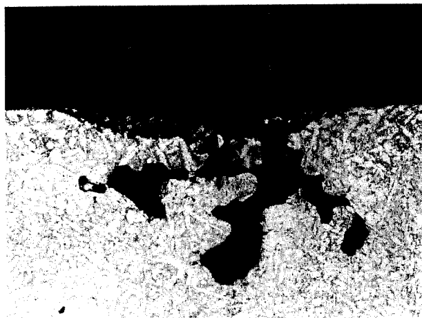
7 Microsection ( \times 50 ) of specimen shown in Fig. 6, etched electrolytically in 1% chromic acid
