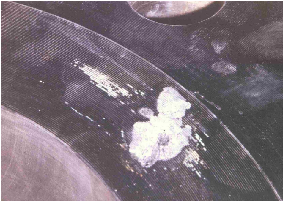
FIGURE 5 - Corrosion of a superduplex flange with a graphite-containing gasket.
