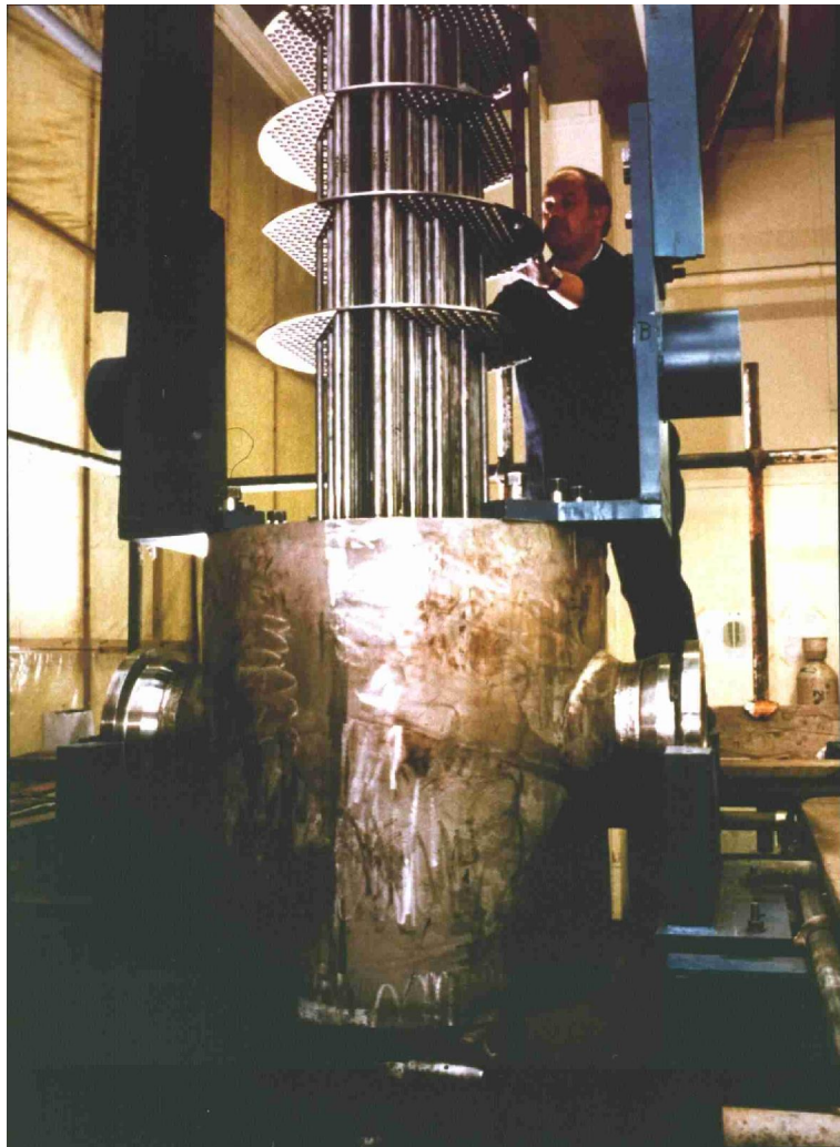
FIGURE 4 High pressure gas cooler with seawater on shell side.
