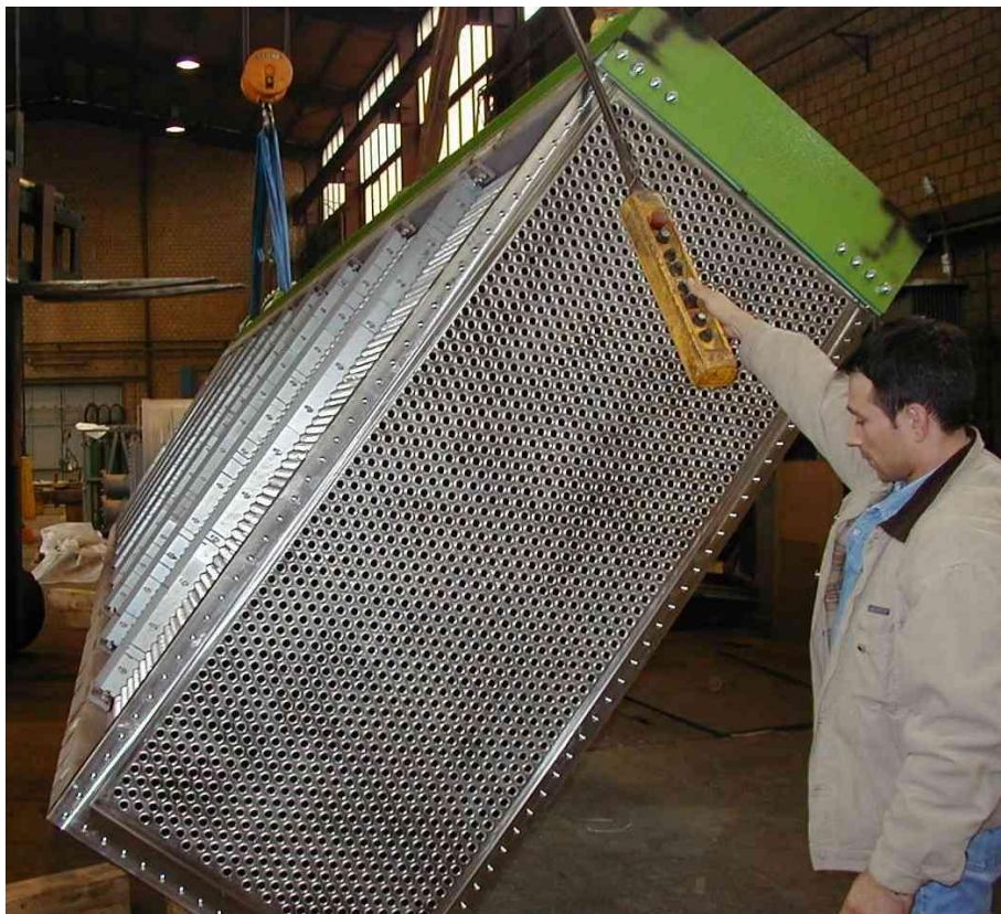
FIGURE 6 Z100 gas cooler for use in seawater with a high solids burden.
