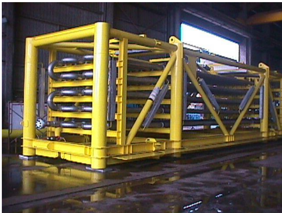
FIGURE 5 Subsea heat exchanger in coated steel frame.
