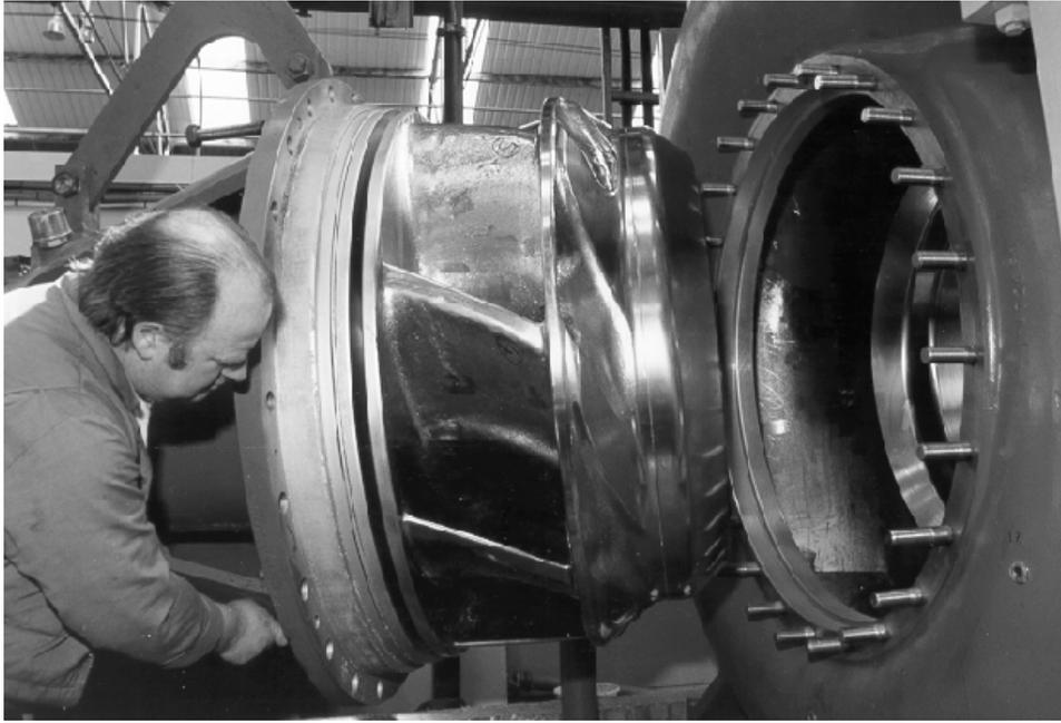
**Figure 7: Z100 slurry recirculation pump fitted at Drax FGD Plant in the UK.**
