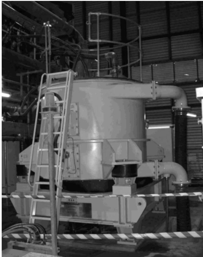
**Figure 8: Z100 centrifuge at Ratcliffe Power Station in the UK.**
