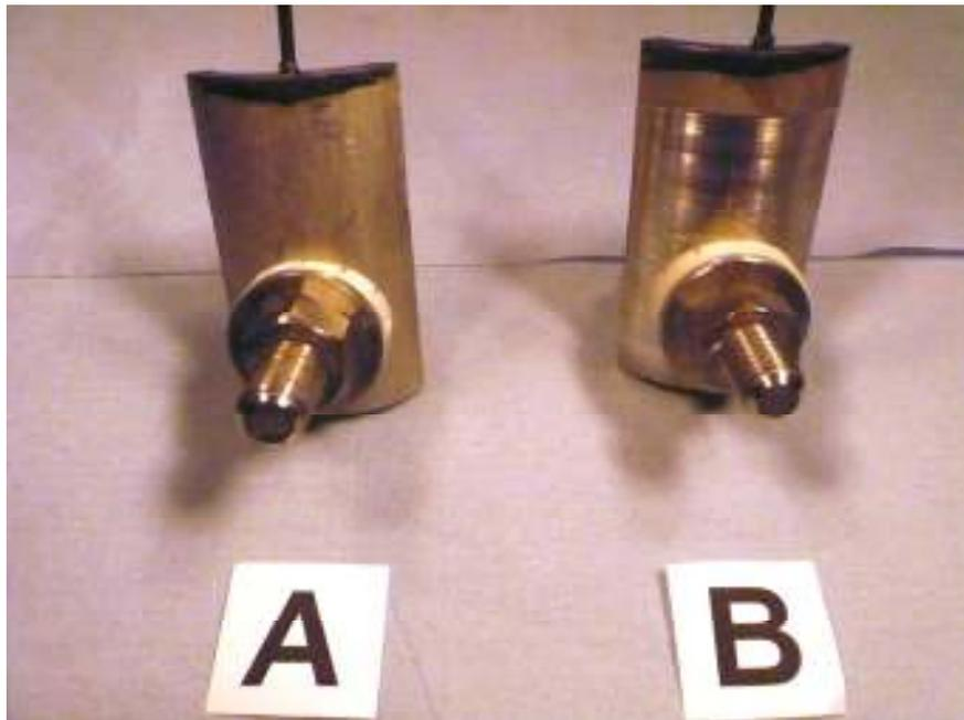
Figure 5 Appearance of creviced pipe sections, A) as received; B) machined.
